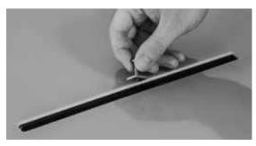
Insert the fin into the SUP's groove and align the bolt's hole with the nut previously installed. Screw lightly and push backwards.
