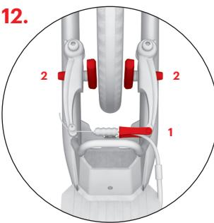
**Adjusting the rear brake** is the same for both models.
