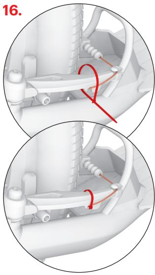
Fasten the end of the brake cable in the lock and secure with the cable tie, then trim the tie.
