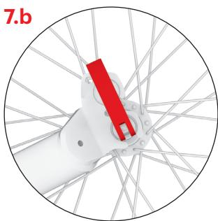
Two-position rear fork enables you to adjust the height of the footrest above the ground. Use the lower position for riding over rough terrain. Close the quick release lever. It should point upwards.
