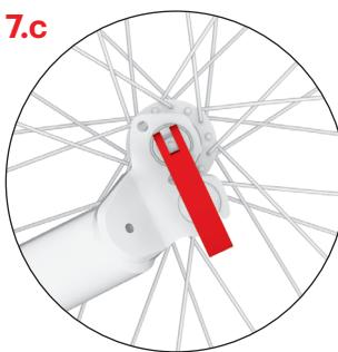
The upper fork position, which reduces the height of the footrest, is designed for riding on a smooth, flat surface. Riding will be less physically demanding. The closed quick release lever should point downwards.
