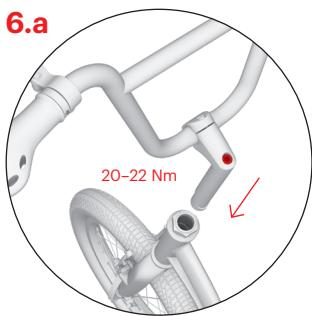
Insert the stem into the frame tube of the scooter and adjust the handlebar height taking care not to position it above the marked line, see pic. 6.b. Make sure that the handlebars are straight and then tighten the screw on the stem.
