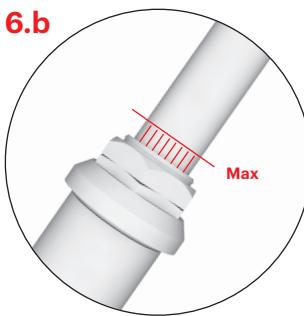
The highest possible height of the handlebars is marked with vertical grooves, at the maximum height the grooves should be visible only partly.
