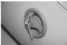
To open the valve for deflation, press down on the valve pin and turn it clockwise so it locks down.
