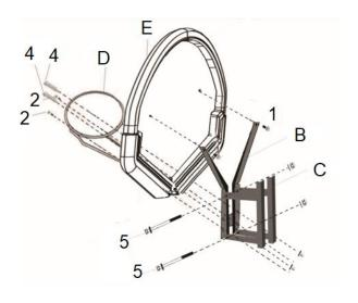
Attach the hoop (D) and the backboard holder (B) to the backboard (E) using bolts (4 and 2). Attach the top part of the backboard holder (B) with bolt (1). Connect the backboard holder (B) to the frame (C) using bolt (5).
