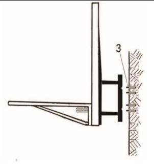
Attach the completed construction to the wall using bolts (3).
