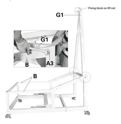
Attach the rear frame G2 to the frame B with 2x bolts A3. Make sure the fixing block on the bottom of the frame face forward.
