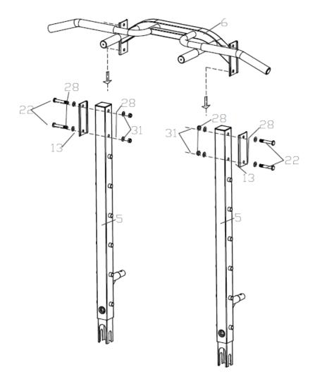
Attach pull up frame (6) to the frames (5) with 4x bolts (22), 8x washers (28), 4x nuts (31) and 2x plates (13).
