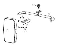
Attach the backrest support (10) to the backrest frame (9) with the knob (17). Attach the backrest (15) to the backrest holder with 4x bolts (27).
