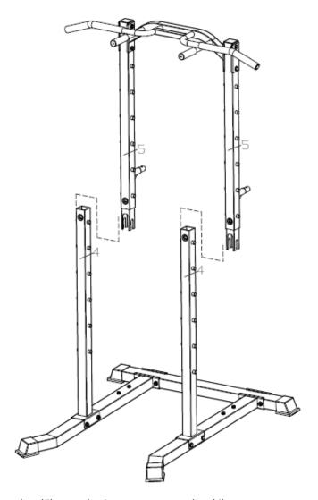
Slide the upper construction (5) onto the bottom construction (4).
