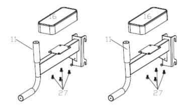
Attach the 2x elbow rests (16) to the handles (11) using the 8x screws (27).
