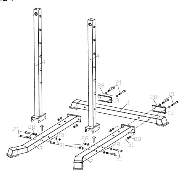
Connect the frames (2 and 3) to the rear frame (1) using 2x plates (13), 8x washers (28), 4x bolts (21) and 4x nuts (31).
