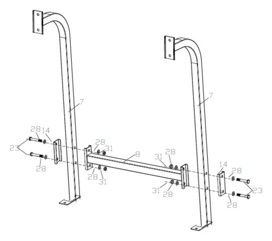
Attach the connection frame (8) to the support frames (7) using 2x plates (14), 4x bolts (23), 8x washers (28) and 4x nuts (31).
