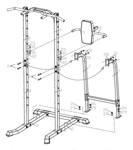
Connect the frames (4 and 5) with the support frames (7) using 4x bolts (24), 4x washers (28) and 4x nuts (31). Fasten the support frames (7) to the stabilizers (2 and 3) using 4x bolts (26) and 4x washers (29). Attach the backrest frame (9) to the frame (5) with 2x bolts (25), 4x washers (30) and 2x nuts (32).
