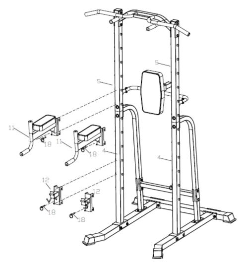
Place the handles (11) on the frames (4 or 5) and secure with the pin (18).
