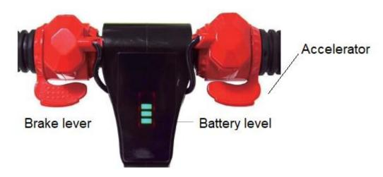
Battery status is displayed in the middle, 4 cells = 100% battery status Control the speed with the accelerator, brake with the brake lever.
