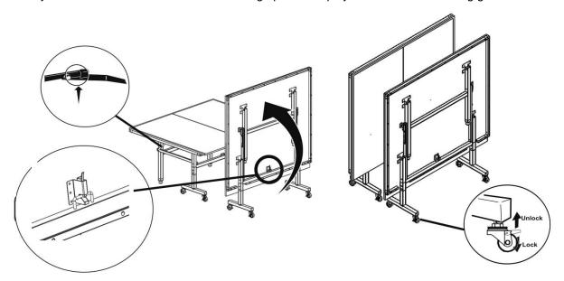
Repeat for the other side of the table, ensure that the table is on an even surface and is stable.
